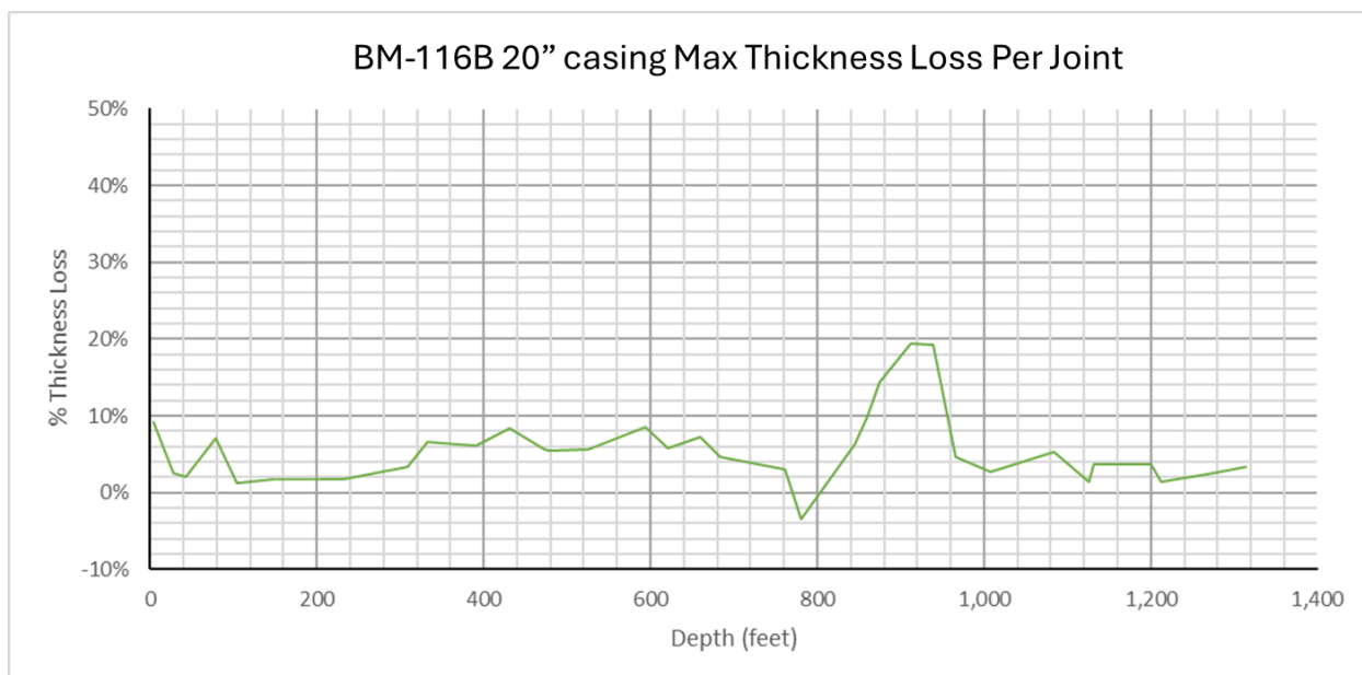
Figure 7. BM-116B pipe thickness loss for the 20" casing
