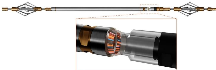
Figure 1: High-resolution acoustic radial imaging tool captures sub-millimetric (0.25 mm) inner casing surface measurements for assessing wall loss defects, breaches, deformation, threaded connection makeup, and completions hardware.
