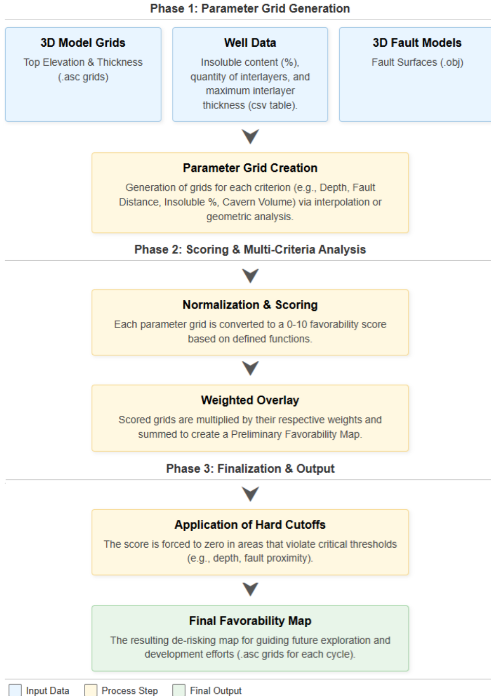
Fig. 6. Schematic description of the favorability mapping algorithm. The workflow is divided into three main stages: (1) generation of spatial parameter grids from various input data; (2) a multi-criteria analysis involving normalization, scoring, and a weighted overlay of the grids; and (3) the application of hard cutoffs to produce the final de-risking map.
