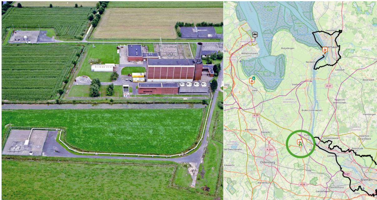
Figure 3: Aerial view of the powerplant and caverns (left, © DEEP.KBB) and location of the powerplant showing the high-voltage lines (purple and yellow) and the gas pipeline (orange) (right, source: https://energy-charts.info/map retrieved on 17.03.2025)
