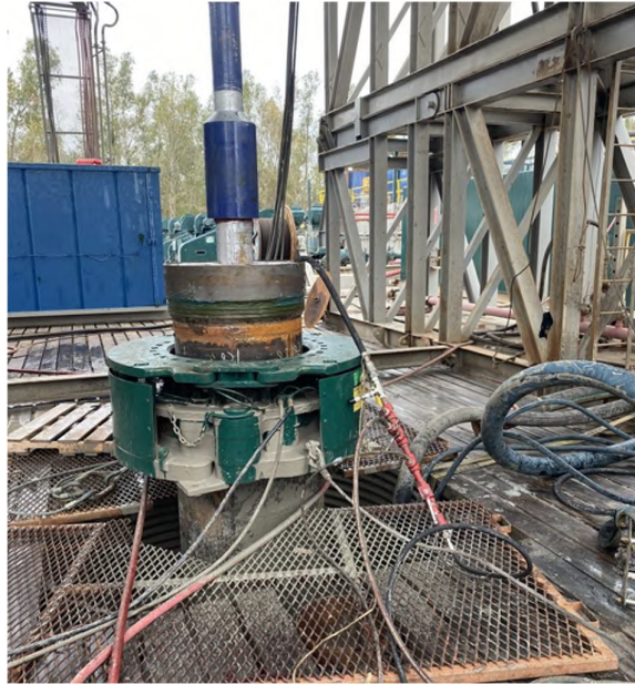
Figure 10 - Pressure Testing Casing Before Running Downhole
