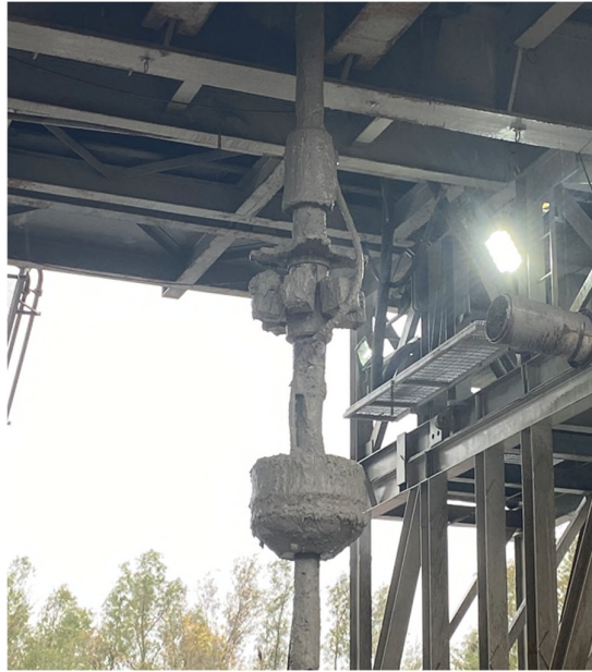
Figure 11 - Cement Laden Spear and Packer Cup After Run
