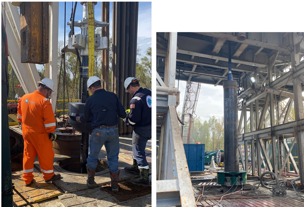
Figure 9 - Deploying Packer Cup and Spear with Liner
