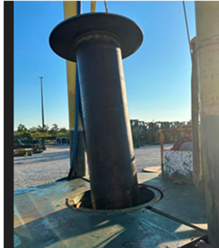
Figure 6 - 30in (76.2cm) Liner Hanger Test Fixture
