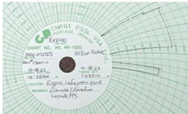
Figure 7 - 800psi (5515.8kPa) pressure test on 30in (76.2cm) Test Casing, Packer Cup and Spear
