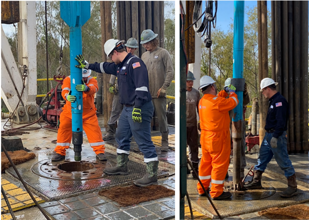
Figure 8 - Deploying Inner-String Latch-In Stinger with Centralizer and SeaCure Slip-Joint Sub
