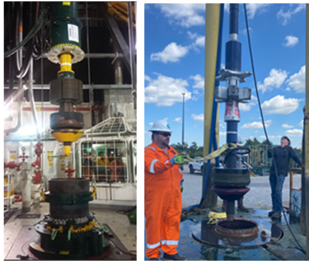
Figure 4 - 30in (76.2cm) CRT Packer Cup Converted to Spear Packer Cup
