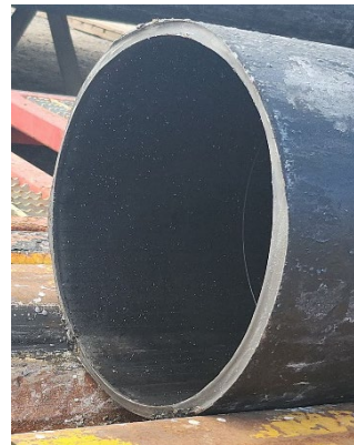
Figure 19. Clean EZ cut of a 13-3/8"
