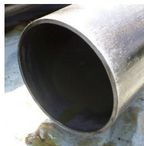
Figure 3. 11-3/4" cut with EZ cutter
